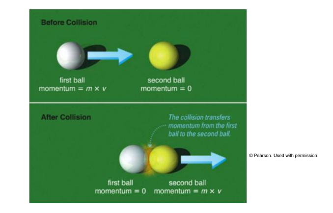
Conservation of momentum (mass × velocity) means an object's momentum cannot change unless it transfers momentum to or from another object. When no force is present, no momentum can be transferred so an object must maintain its speed and direction.
